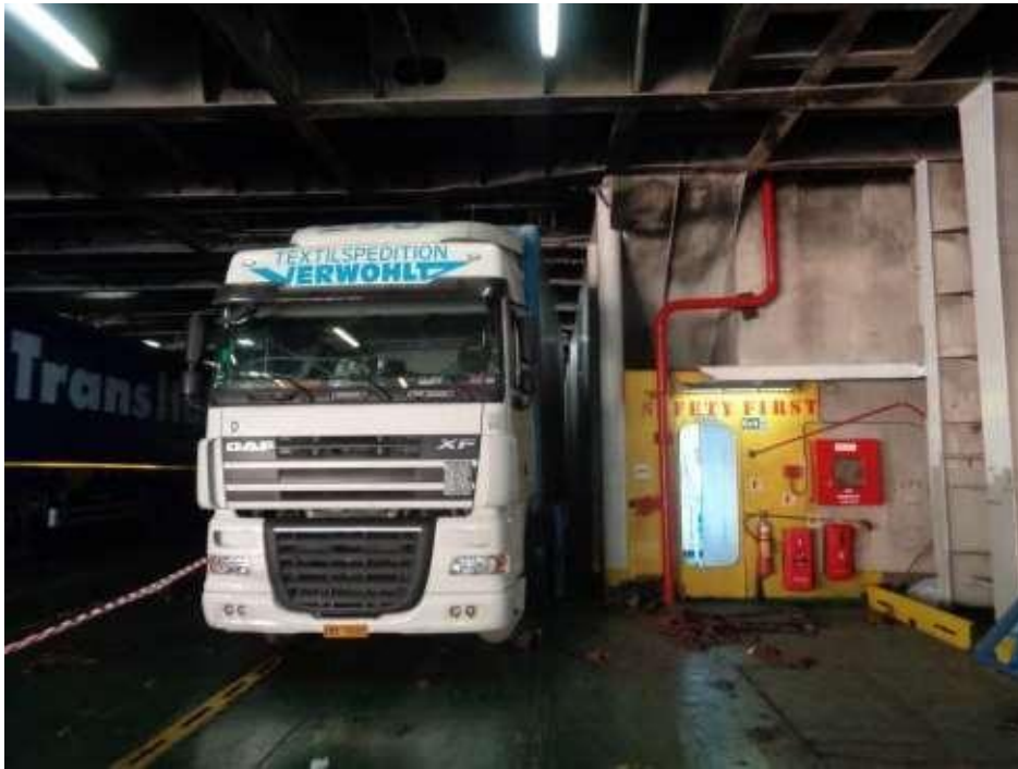
Figure 5: The rigid truck parked next to the engine room entrance bulkhead after the accident.
