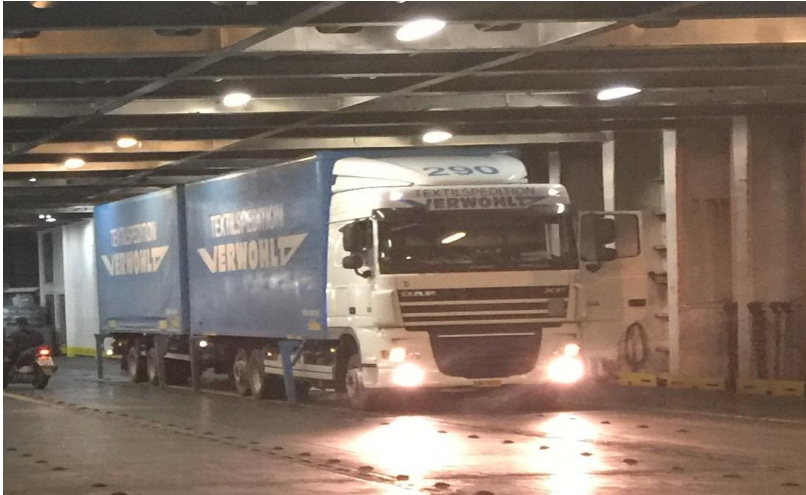
Figure 3: The rigid truck with drawbar trailer involved in the marine casualty. All supporting legs of the right trailer's side are lowered. Photo taken during the reconstruction of the accident.
