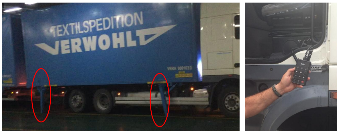
Figure 6. The two supporting legs fitted on the first trailer's outer side and the cabled remote control for the operation of the chassis' air suspension system.
