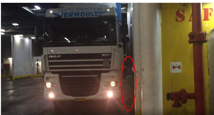
Figure 8: Estimated position of the driver trapped between the trailer and the bulkhead. Photo taken during the reconstruction of the accident.
