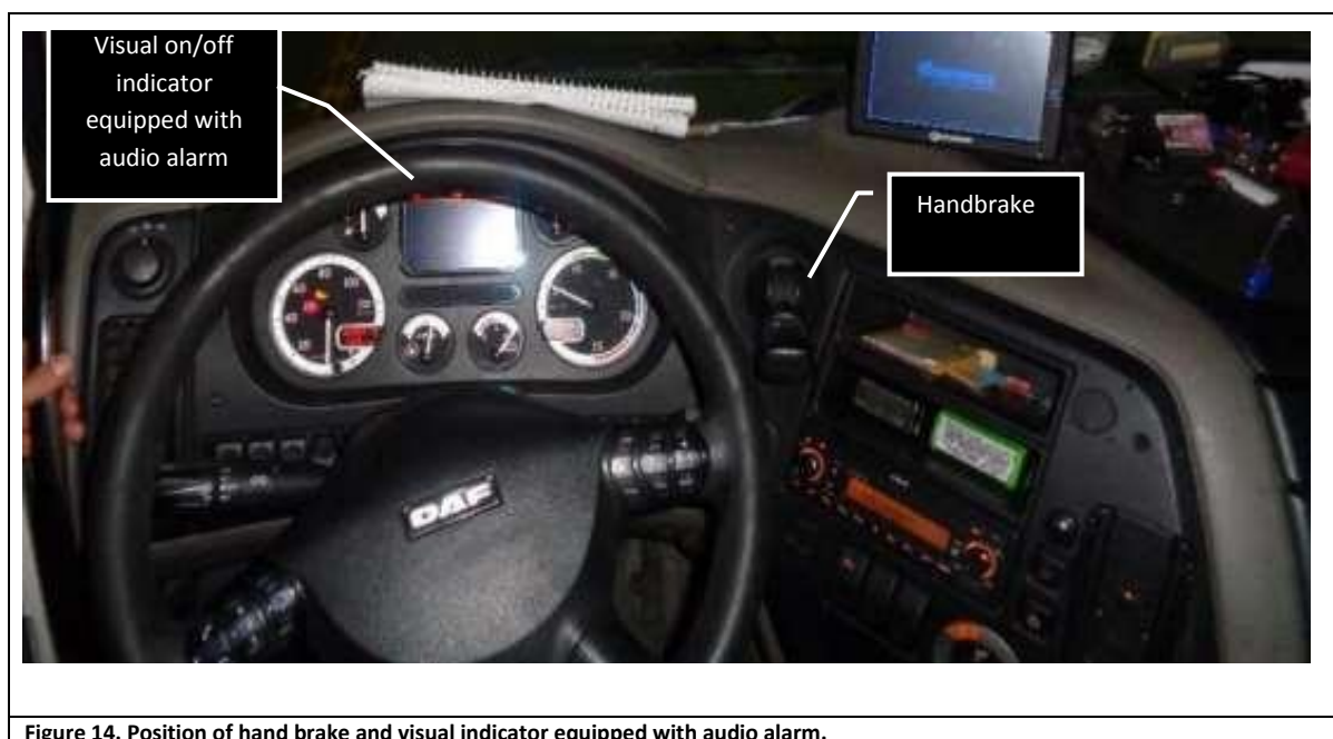
Figure 14. Position of hand brake and visual indicator equipped with audio alarm.
