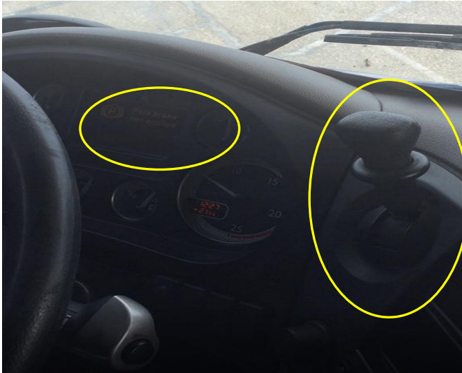
Figure 9: The parking brake lever and the visual indication on tractor cockpit.
