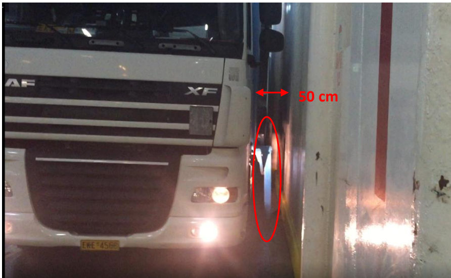
Figure 7: The space formed between the truck trailers and the engine room entrance bulkhead. Photo taken during the reconstruction of the accident.
